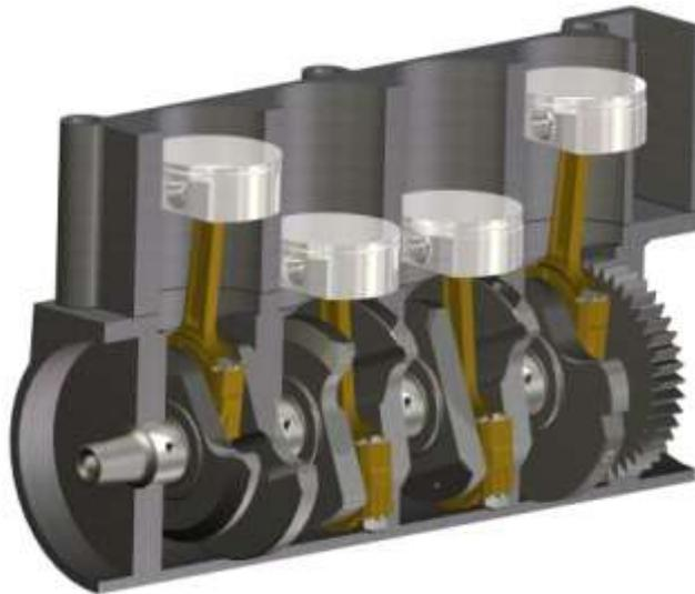
Figure 1: CAD model of Yamaha YZF-R1 Motorcycle Engine
